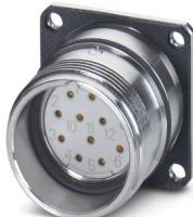
M23, Device connector front mounting, series: RC, straight, Screw locking mechanism, Direction of rotation: Standard, contact connection type: Socket, Solder-in connection, Flat gasket, Panel thickness min.: 2.7 mm, Panel thickness max.: 3.5 mm, coding: N. This product is in the process of being discontinued. This product must no longer be considered for new projects. Please contact your sales representative for alternatives.
