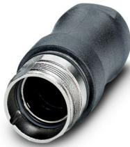
Housing for circular connector, series: RC, straight plastic-sheathed, Screw locking mechanism, M23, number of positions: 12, contact connection type: Socket, Crimp connection, shielded: yes, cable diameter range: 2 mm... 10.5 mm. This product is in the process of being discontinued. This product must no longer be considered for new projects. Please contact your sales representative for alternatives.
