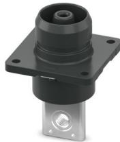
Connector, color: black, number of positions: 1, min. conductor cross-section: 95 mm<sup>2</sup>, max. conductor cross-section: 120 mm<sup>2</sup>, rated voltage: 1500 V DC, rated current: 350 A, Connection method: Thread connection
