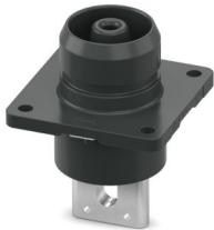
Connector, color: black, number of positions: 1, min. conductor cross-section: 95 mm<sup>2</sup>, max. conductor cross-section: 120 mm<sup>2</sup>, rated voltage: 1500 V DC, rated current: 350 A, Connection method: Thread connection
