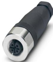
Connector, Universal, 4-position, Socket straight M12, coding: A, Screw connection, knurl material: Stainless steel 1.4404, cable gland Pg7, external cable diameter 4 mm ... 6 mm
