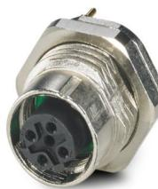
Device connector rear mounting, Ethernet, 4-position, Socket, straight, M12-SPEEDCON, D-coding, Wave soldering, this item is expected to be lead-free from Q2 2026 in accordance with RoHS II without exception 6c (Pb < 0.1%), a lead-free alternative is possible on request in advance
