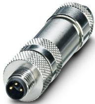
Connector, Universal, 3-position, shielded, Plug straight M8, coding: A, Screw connection, knurl material: Brass, nickel-plated, external cable diameter 3.5 mm ... 5.5 mm
