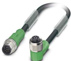
Sensor/actuator cable, 8-position, PUR halogen-free, black-gray RAL 7021, Plug straight M12, coding: A, on Socket angled M12, coding: A, cable length: 1.5 m
