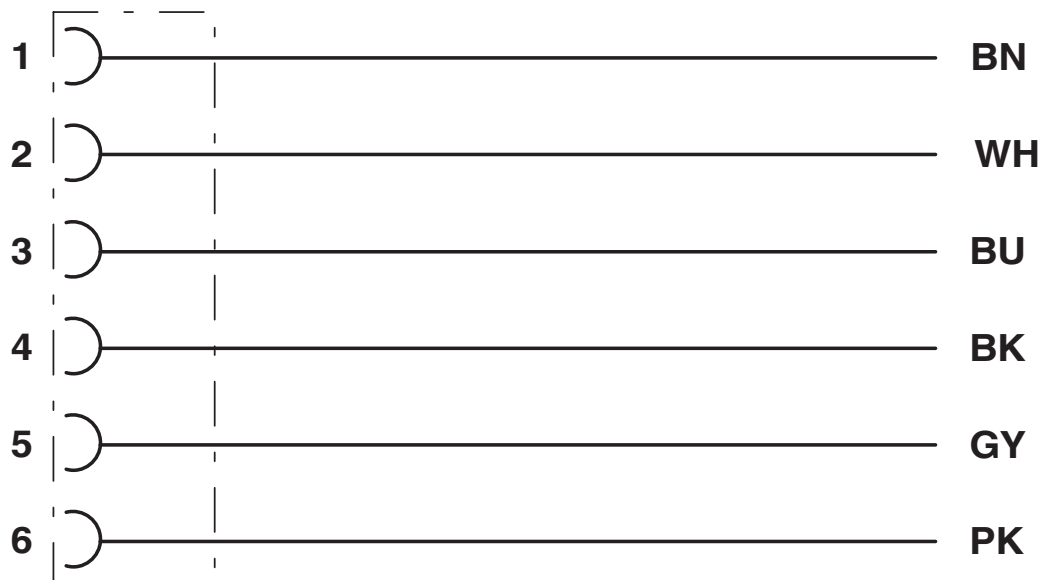
Contact assignment of M8 socket
