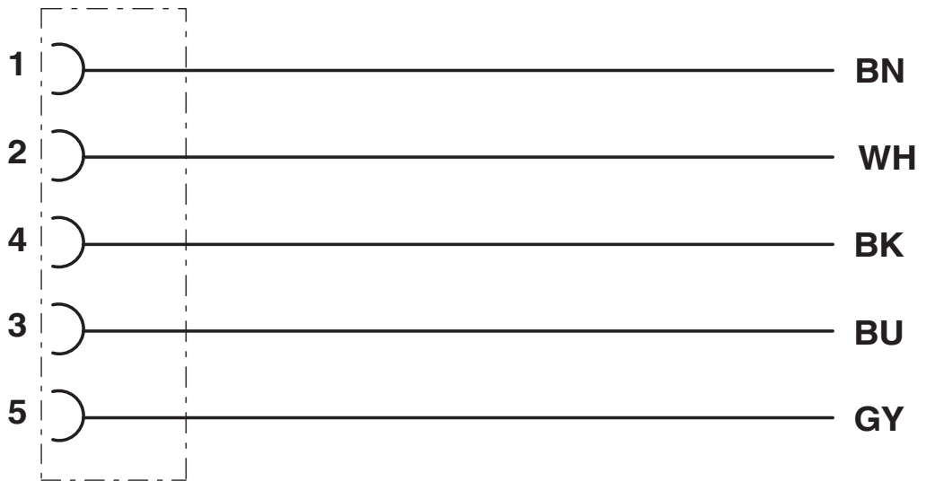
Contact assignment of the M12 socket
