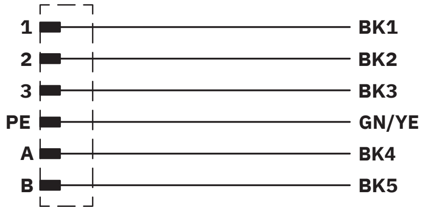
Contact assignment of the M15 connector
