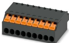
PCB connector, nominal cross section: 1.5 mm<sup>2</sup>, color: black, nominal current: 8 A, rated voltage (III/2): 160 V, contact surface: Sn, contact connection type: Socket, number of rows: 1, number of positions: 9, product range: XPC 1,5/..-ST, pitch: 3.5 mm, connection method: Push-X-connection, conductor/PCB connection direction: 0 °, locking clip: - without locking clip, plug-in system: COMBICON MC 1,5, locking: without, mounting method: without, type of packaging: packed in cardboard
