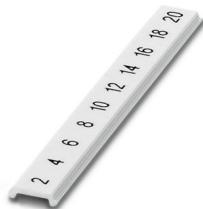
Zack Marker strip, flat, Strip, white, labeled, printed horizontally: consecutive even numbers 2 ... 20, 22 ... 40, etc. up to 82 ... 100, mounting type: latching, for terminal block width: 5 mm, Number of individual labels: 10, text field height: 5.15 mm, text field width: 5.15 mm
