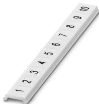
Zack Marker strip, flat, Strip, white, labeled, printed horizontally: consecutive numbers 1 ... 10, 11 ... 20, etc. up to 491 ... 500, mounting type: latching, for terminal block width: 5 mm, Number of individual labels: 10, text field height: 5.15 mm, text field width: 5.15 mm
