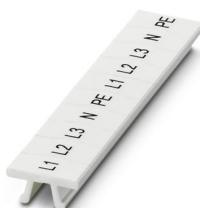
Zack marker strip, Strip, white, labeled, horizontal: L1, L2, L3, N, PE, L1, L2, L3, N, PE, mounting type: latching, for terminal block width: 5.2 mm, Number of individual labels: 10, text field height: 10.5 mm, text field width: 5.15 mm
