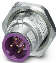
Device connector rear mounting, 5-position, Pin, straight, M12-SPEEDCON, B-coding, Wave soldering, this item is expected to be lead-free from Q1 2026 in accordance with RoHS II without exception 6c (Pb < 0.1%), a lead-free alternative is possible on request in advance
