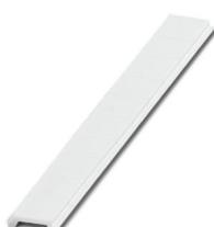
Zack Marker strip, flat, can be ordered: Strip, white, labeled according to customer specifications, mounting type: snap into flat marker groove, for terminal block width: 5 mm, Number of individual labels: 10, text field height: 5.15 mm, text field width: 5.15 mm
