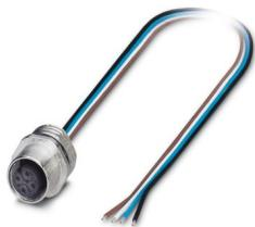
Device connector front mounting, 5-position, Socket, straight, M12, A-coding, Individual wires, cable length: 0.8 m, 0.34 mm<sup>2</sup>, TPE litz wire, potted
