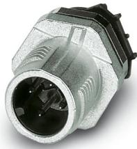
Sensor/actuator flush-type connector, connector, 4-pos., M12 SPEEDCON, A-coded, rear/screw mounting with M12 thread, with straight THR solder connection
