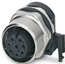
Device connector front mounting, 8-position, Socket, angled, M12-SPEEDCON, A-coding, THR and wave soldering, this item is expected to be lead-free from Q2 2026 in accordance with RoHS II without exception 6c (Pb < 0.1%), a lead-free alternative is possible on request in advance
