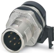
Device connector rear mounting, 8-position, Pin, angled, M12-SPEEDCON, A-coding, THR and wave soldering, this item is expected to be lead-free from Q2 2026 in accordance with RoHS II without exception 6c (Pb < 0.1%), a lead-free alternative is possible on request in advance
