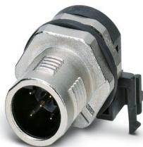
Device connector rear mounting, 5-position, Pin, angled, M12-SPEEDCON, B-coding, THR and wave soldering, this item is expected to be lead-free from Q2 2026 in accordance with RoHS II without exception 6c (Pb < 0.1%), a lead-free alternative is possible on request in advance
