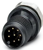
Sensor/actuator flush-type connector, socket, 8-pos., M12, A-coded, front/screw mounting with M12 thread, with solder cups, plastic version
