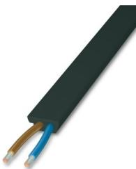
AS-Interface EPDM flat conductor in black, for additional power supply, 2 x 1.5 mm<sup>2</sup>, 1000 m on a disposable drum
