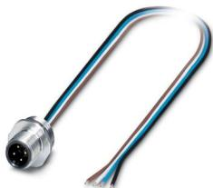
Device connector front mounting, 3-position, Pin, straight, M12-Standard, A-coding, on free cable end, Individual wires, cable length: 0.5 m, 0.34 mm<sup>2</sup>, TPE litz wire, potted, this item is expected to be lead-free from Q4 2025 in accordance with RoHS II without exception 6c (Pb < 0.1%), a lead-free alternative is possible on request in advance
