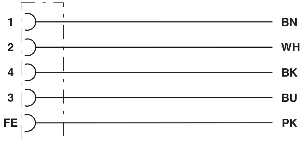
Contact assignment of the M12 socket
