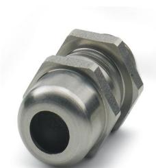
Cable gland, material for screw connection: Stainless steel 1.4305, application: Standard, external cable diameter 6 mm ... 12 mm, shielding: no, connecting thread: M20 x 1.5, color: silver-colored, with O-ring
