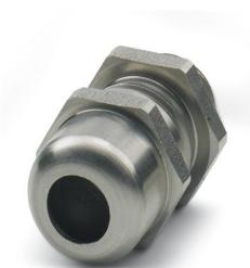
Cable gland, material for screw connection: Stainless steel 1.4305, application: Standard, external cable diameter 5 mm ... 10 mm, shielding: no, connecting thread: M16 x 1.5, color: silver-colored, with O-ring
