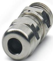
Cable gland, material for screw connection: Brass, nickel-plated, application: Standard, external cable diameter 4 mm ... 7 mm, shielding: no, connecting thread: M16 x 1.5, color: silver-colored, with pressure compensation element and O-ring
