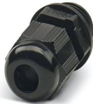
Cable gland, material for screw connection: PA, application: Standard, external cable diameter 4 mm ... 7 mm, shielding: no, connecting thread: M16 x 1.5, color: jet black RAL 9005, with pressure compensation element and flat gasket
