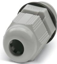
Cable gland, material for screw connection: PA, application: Standard, external cable diameter 6 mm ... 11 mm, shielding: no, connecting thread: M20 x 1.5, color: lightgray RAL 7035, with pressure compensation element and flat gasket
