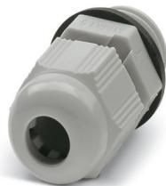
Cable gland, material for screw connection: PA, application: Standard, external cable diameter 4 mm ... 7 mm, shielding: no, connecting thread: M12 x 1.5, color: lightgray RAL 7035, with pressure compensation element and flat gasket
