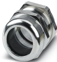
Cable gland, material for screw connection: Brass, nickel-plated, application: Standard, external cable diameter 22 mm ... 32 mm, shielding: no, connecting thread: M50 x 1.5, color: silver-colored, with O-ring
