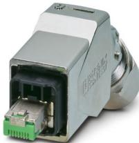
RJ45 connector, degree of protection: IP65/IP67, number of positions: 8, 1 Gbps, CAT5 (IEC 11801:2002), material: Metal, connection method: IDC fast connection, connection cross section: AWG 26- 24, cable outlet: angled
