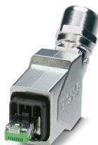
Push-pull connector (version 14), die-cast zinc, with RJ45 connector insert, 8-pos., with IDC fast connection technology, for 1 and 7-wire cores, 23 ... 22 AWG, for cable diameter of 5.5 mm ... 10 mm
