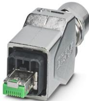
RJ45 connector, degree of protection: IP65/IP67, number of positions: 8, 1 Gbps, CAT5 (IEC 11801:2002), material: Metal, connection method: IDC fast connection, connection cross section: AWG 23- 22, cable outlet: straight
