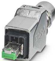
RJ45 connector, degree of protection: IP65/IP67, number of positions: 8, 1 Gbps, CAT5, material: Metal, connection method: IDC fast connection, connection cross section: AWG 26- 24, cable outlet: straight, Ethernet
