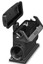
Surface mounting housing B24, with single locking latch, material: PA 6.6-FR, protective cover material: PC, cable outlets: 2, lateral, 2x M32, height: 84 mm, cable gland: none, protective cover: yes, Standard, including 2x reducing adapter
