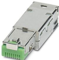
RJ45 male insert, design: RJ45, degree of protection: IP20, number of positions: 8, 1 Gbps, CAT5 (IEC 11801:2002), material: Metal, connection method: Insulation displacement connection, connection cross section: AWG 23- 22, cable outlet: straight, Ethernet/PROFINET
