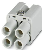
Contact insert, number of positions: 4, size: D7, number of connections per position: 1, Socket, Crimp connection, 830 V, 40 A, 1.5 mm<sup>2</sup> ... 6 mm<sup>2</sup>, application: Power, Only suitable for plastic housings, four coding options
