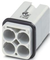
Contact insert, number of positions: 4, size: D7, number of connections per position: 1, Pin, Crimp connection, 830 V, 40 A, 1.5 mm<sup>2</sup> ... 6 mm<sup>2</sup>, application: Power, Only suitable for plastic housings, four coding options
