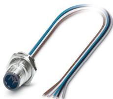
Device connector rear mounting, Universal, 5-position, Pin, straight, M12-Standard, B-coding, on free cable end, Individual wires, cable length: 0.5 m, 0.34 mm<sup>2</sup>, TPE litz wire, potted, this item is expected to be lead-free from Q1 2026 in accordance with RoHS II without exception 6c (Pb < 0.1%), a lead-free alternative is possible on request in advance
