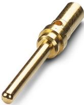
D-SUB crimp contact, series: HC-M-DSUB-C, Pin, turned, contact diameter: 1 mm, rated current: 5 A, connection cross section: 0.08 mm<sup>2</sup> ... 0.12 mm<sup>2</sup>, AWG 28...24, contact material: Metal
