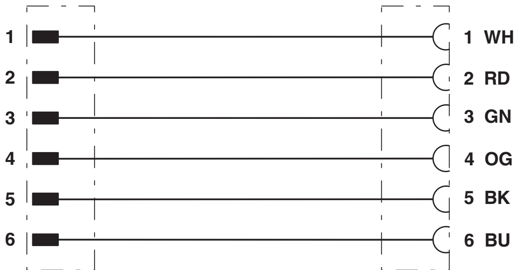
Contact assignment of 7/8" plugs/sockets
