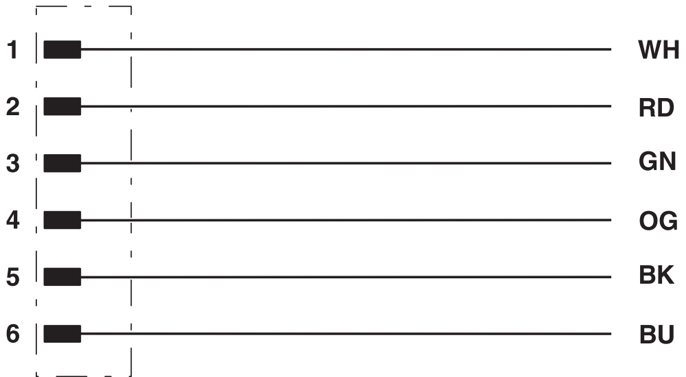
Contact assignment of 7/8" plug
