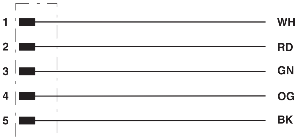
Contact assignment of 7/8" plug
