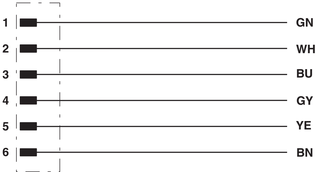
Contact assignment of 7/8" plug
