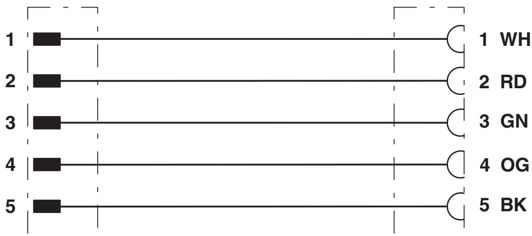
Contact assignment of 7/8" plugs/sockets
