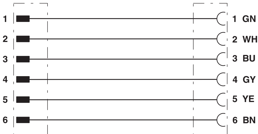
Contact assignment of 7/8" plugs/sockets
