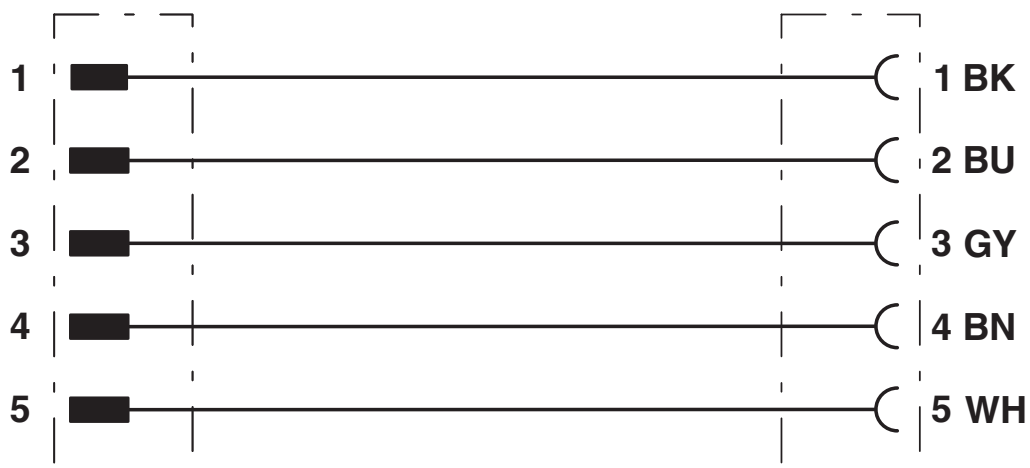
Contact assignment of 7/8" plugs/sockets
