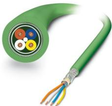
By the meter, Data cable, PROFINET CAT5 (100 Mbps), EtherCAT® CAT5 (100 Mbps), shielded, PUR halogen-free, green RAL 6018, 4-wire (1x4xAWG22/19, S/TQ), color single wire: white, yellow, blue, orange, cable length: 100 m
